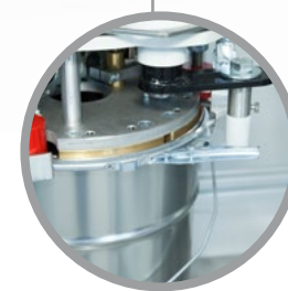
Station 3 Clamping ring is closed
