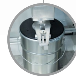
Station 2 Clamping ring is placed into the closing position
